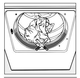
Important: Please check that items of laundry cannot be trapped by the door, as this will cause damage to the fabric.
